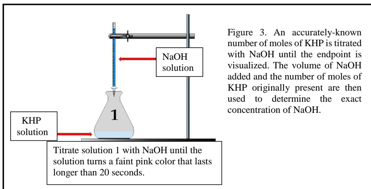
Figure 3. An accurately-known number of moles of KHP is titrated with NaOH until the endpoint is visualized. The volume of NaOH added and the number of moles of KHP originally present are then used to determine the exact concentration of NaOH.
