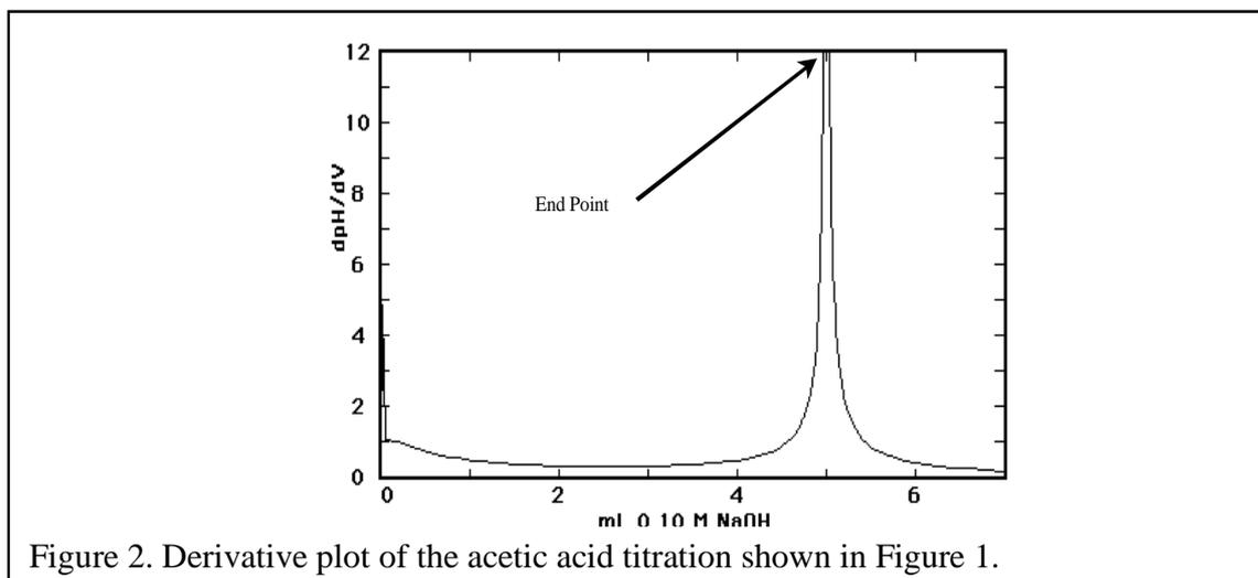
The derivative of the titration curve is approximated by the finite differences:
