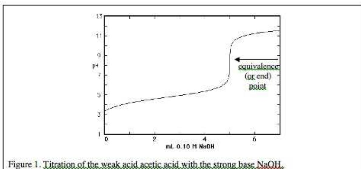
The equivalence point (or the end point) of the titration can be estimated visually, as in Figure 1. A more accurate approach is to calculate the derivative ( $d\text{pH}/dV$ ) of the titration curve and plot this function versus volume of added base. As shown in Figure 2, the derivative plot exhibits a clear maximum at the equivalence point.
