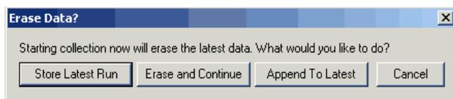
To overlay the next spectrum on top of the last spectra, click on Store Latest Run.
