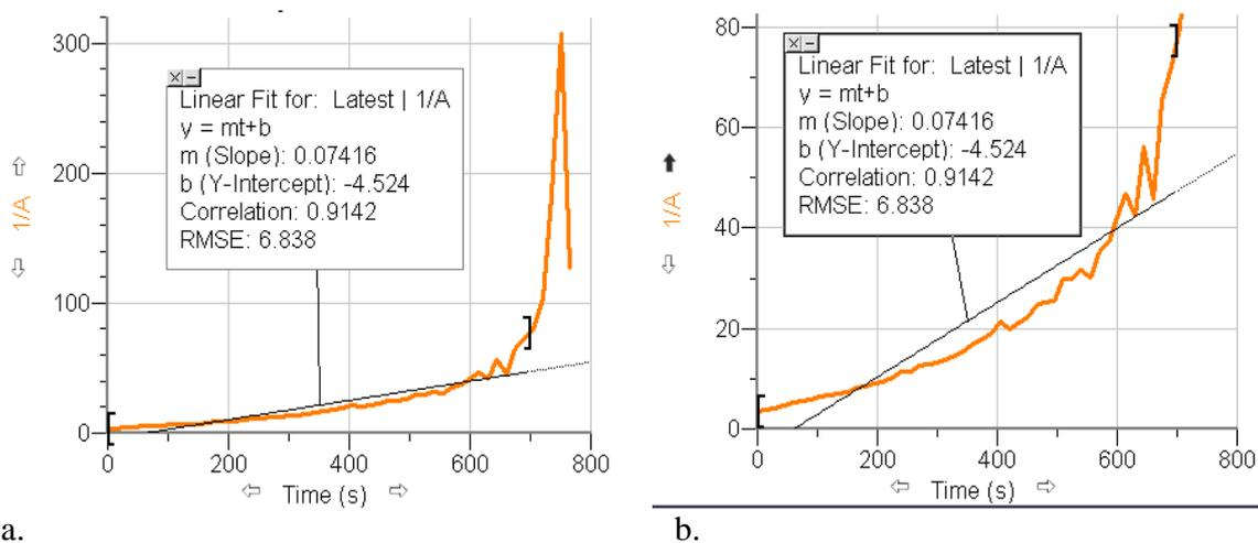
Figure 11. (a.) The y-axis range is too large because of noisy points at the long-time end. (b.) Expand the y-axis scale to get a comparable view to the  $\ln A$  vs. t plot (compare with Figure 9 at right).
