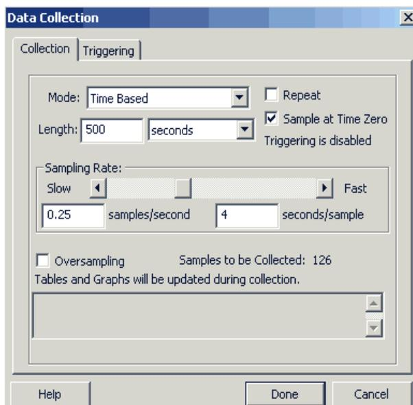
Figure 7. Setting the sampling time interval and total experiment length.
