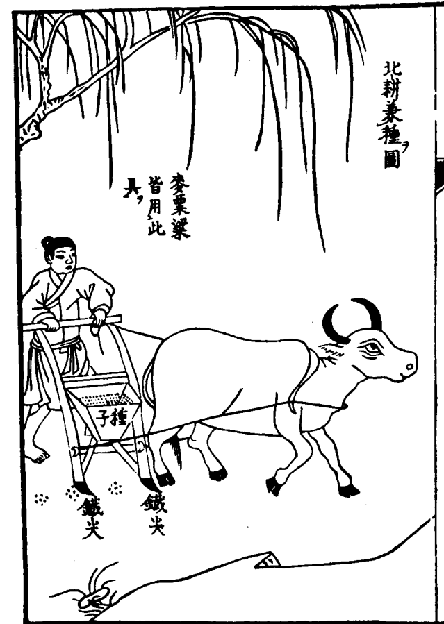
Figure 41. Chinese seed-drill used for sowing cereals, from the Thien Kung Khai Wu (Exploitation of the Works of Nature), 1637.
