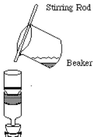
**Figure 2. Pouring down a stirring rod.**
