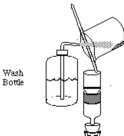
**Figure 3. Washing the precipitate into the Gooch crucible.**
