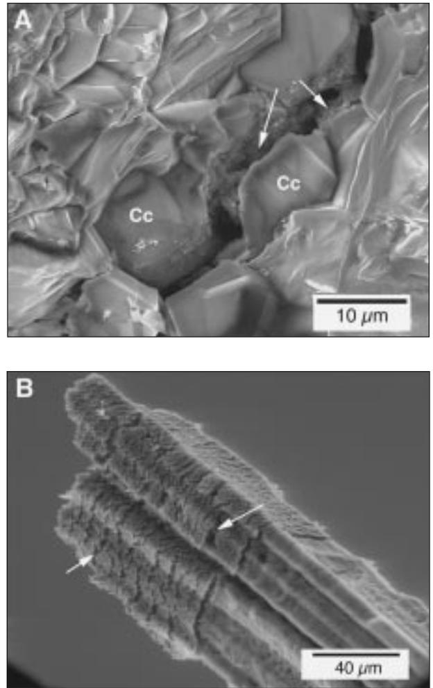
**Figure 5.** Mirabilite crystals developed: (A) generating fractures within the sparitic calcite cement (Cc) of the limestone on the wind-exposed face and transformed to thenardite (arrows) through a dehydration process occurring after mirabilite crystallization and growth; and (B) mirabilite efflorescence (whiskers) on the nonexposed face (arrows indicate incipient dehydration areas).
