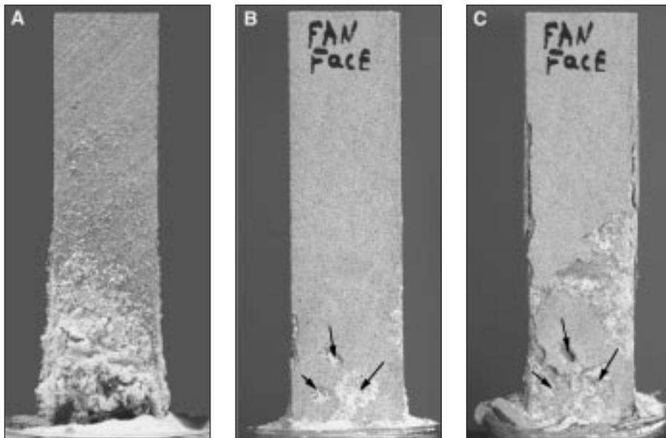
Figure 3. (A) Massive salt efflorescence growth on the non-wind-exposed face six days after the start of the experiment. (B, C) Incipient alveoles (arrows) formation on the wind-exposed face of oolitic limestone slabs after 6 (left) and 28 (right) days. Samples tested in the laboratory at Getty Conservation Institute, Los Angeles, California.
