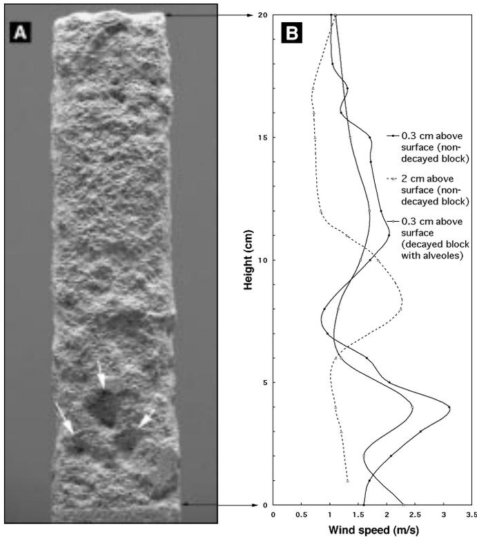
**Figure 4.** (A) Final appearance of the wind-exposed surface after decay test completion, correlated with (B) wind speed measured 0.3 cm (solid lines) and 2 cm (dotted line) from the surface. Note that maximum wind speed at the surface corresponds with maximum decay and alveoles (arrows) development on the bottom part of the stone block.
