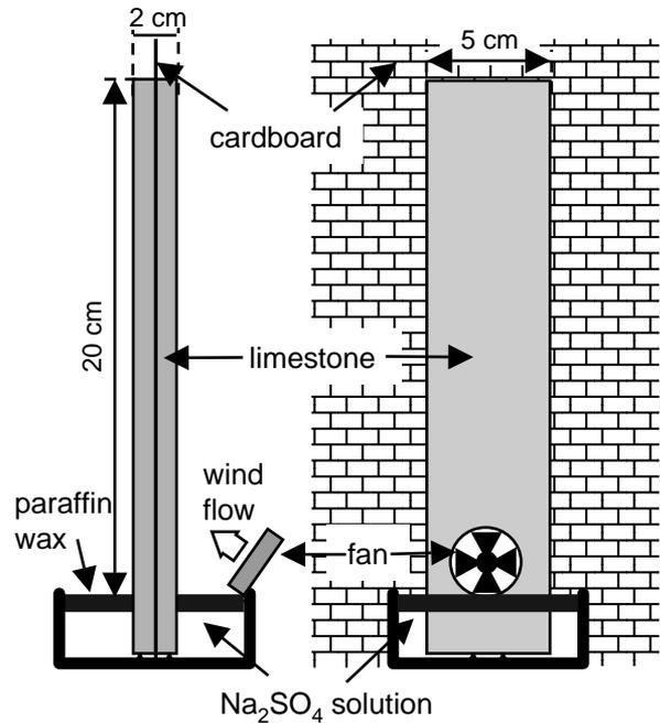
Figure 2. Lateral (left) and frontal (right) view of the salt decay test experimental design.
